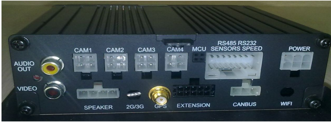
Pic 8 Back Panel interface definition
