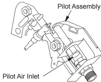
**Figure 25 - Pilot Inlet Air (Propane/LP Pilot Shown)**
