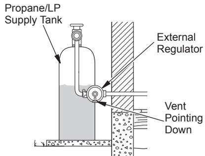
**Figure 14 - External Regulator With Vent Pointing Down**
