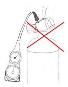
5. Never over-flex your hose. Never fold the hose back onto itself. If your hose is too long, you may loop it and secure it in place with a section of rubber tubing (such as the inner tube of a bicycle tire). However, the minimum bending radius must be at least 3.5 times the outer diameter of the hose. For example, if the outer diameter of your hose is 8mm, then the minimum bending radius (as measured to the inside of the hose) is 28 mm.
