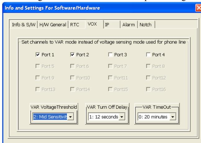
If you connect any of the **TeleCorder** inputs to audio sources that do not have standard on-hook/off-hook voltages, these channels must be set for audio or voice activated recording (**VAR**).
