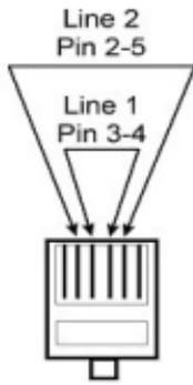
Two T-12 cables (12' phone line cable with T-adapter, photo at right) are supplied with the recorder. You can use these or other suitable cables to connect to your phone lines or other
