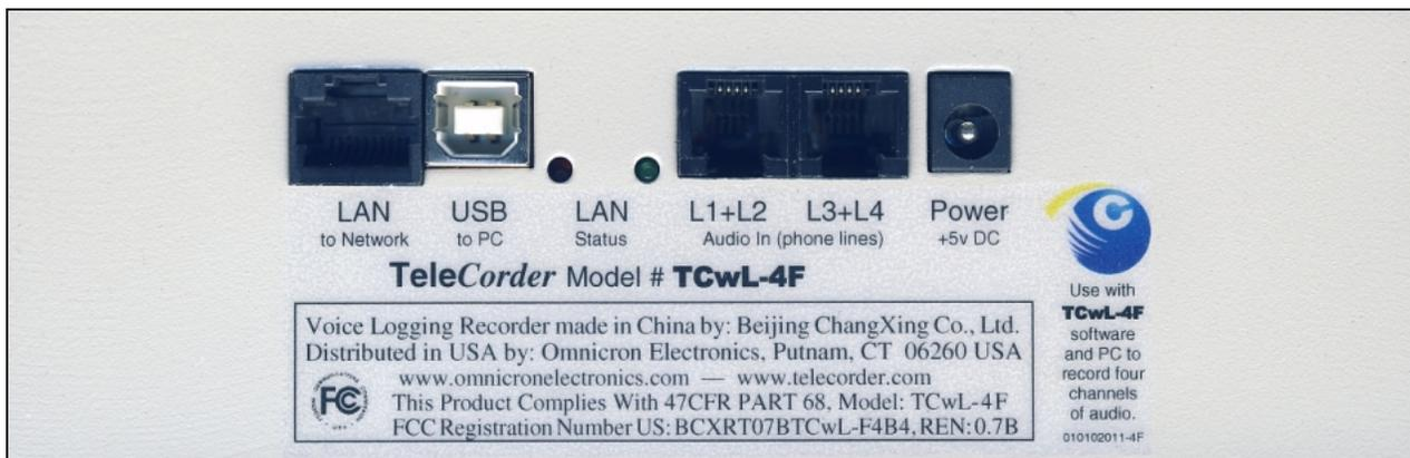
Rear view, LAN and USB jacks for remote access to recordings and configuring via PC, red LAN connection LED, green LAN activity LED, two modular input jacks for connecting to the sources of the conversations to be recorded (two channels per jack with four channel TCwL-4F), and +5vDC input jack for use with the supplied AC adapter.
