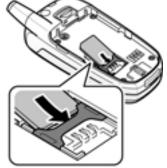
When you need to remove the SIM card, slide it upwards, as shown, and take it out of the socket.
