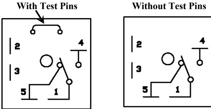
The agitation timer is standard equipment for the floor standing dispenser. The purpose of the timer is to periodically agitate the ice in the bin to prevent congealing. Non adjustable timers with test pins are used on all current production models.
