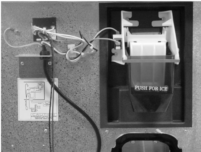
The agitation timer is located at the front of the dispenser on the left side of the ice chute.
