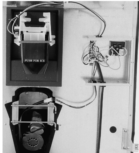
The agitation timer is located in the electrical box at the front of the dispenser. The drawing shows the position of the dials when the timer is set correctly.
