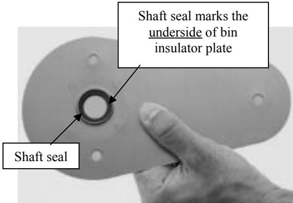
**5** Locate the shaft seal on the underside of the bin insulator plate.
