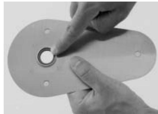
**7** With the convex side of the shaft seal facing up (and the concave, ridge side facing down), snap the new shaft seal onto the bin insulator plate.
