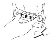
► Take out the motor protection filter and the odor filter out of the filter grip.
