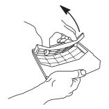
➤ Take out the filter lock by pressing the open endings together.
