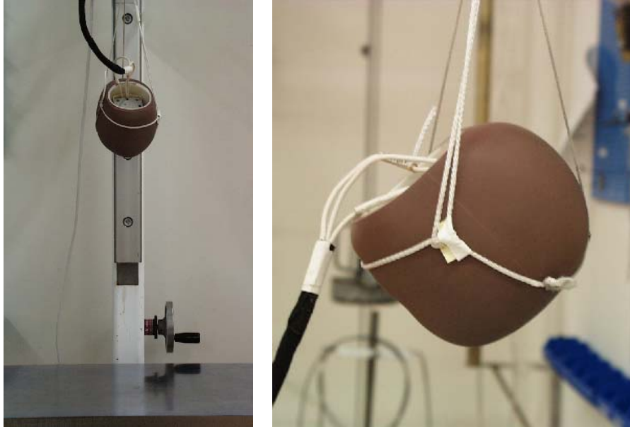
Figure 16: Head drop table test set-up and Q0 child dummy head in harness (pictures do not show correct drop height and drop angle)
