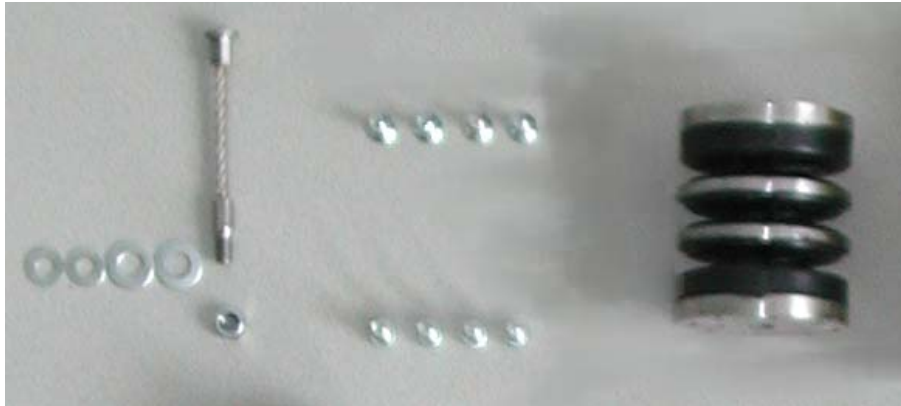
Figure 5: Q0 child dummy neck - neck moulded rubber with two end plates and two intermediate disks, neck cable with washers and nut and two sets of interface attachment bolts.
