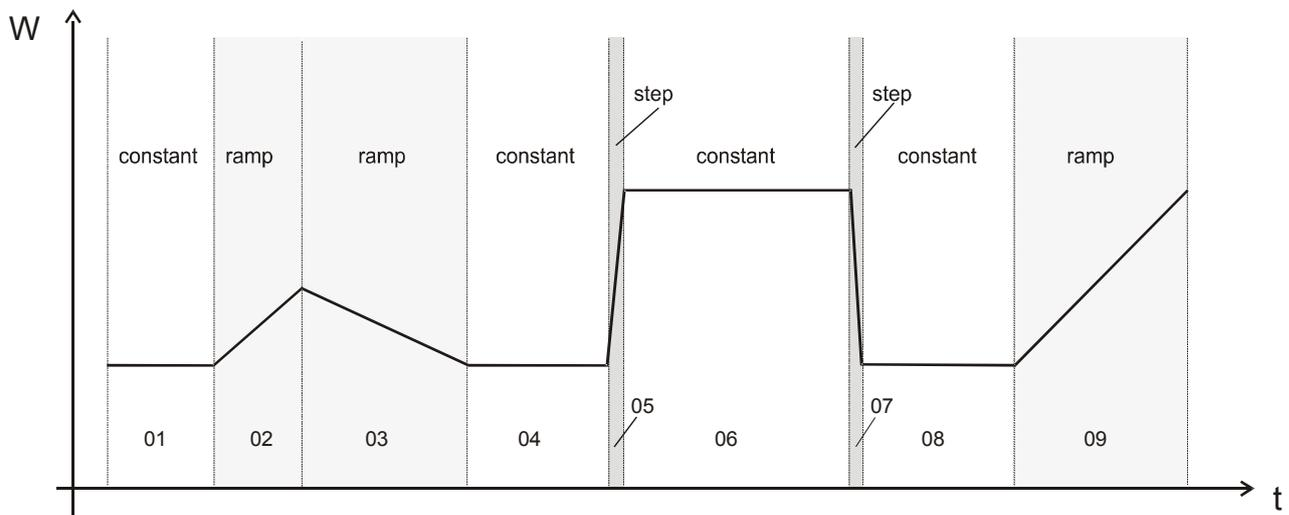
Figure 7: Possible temperature transitions
