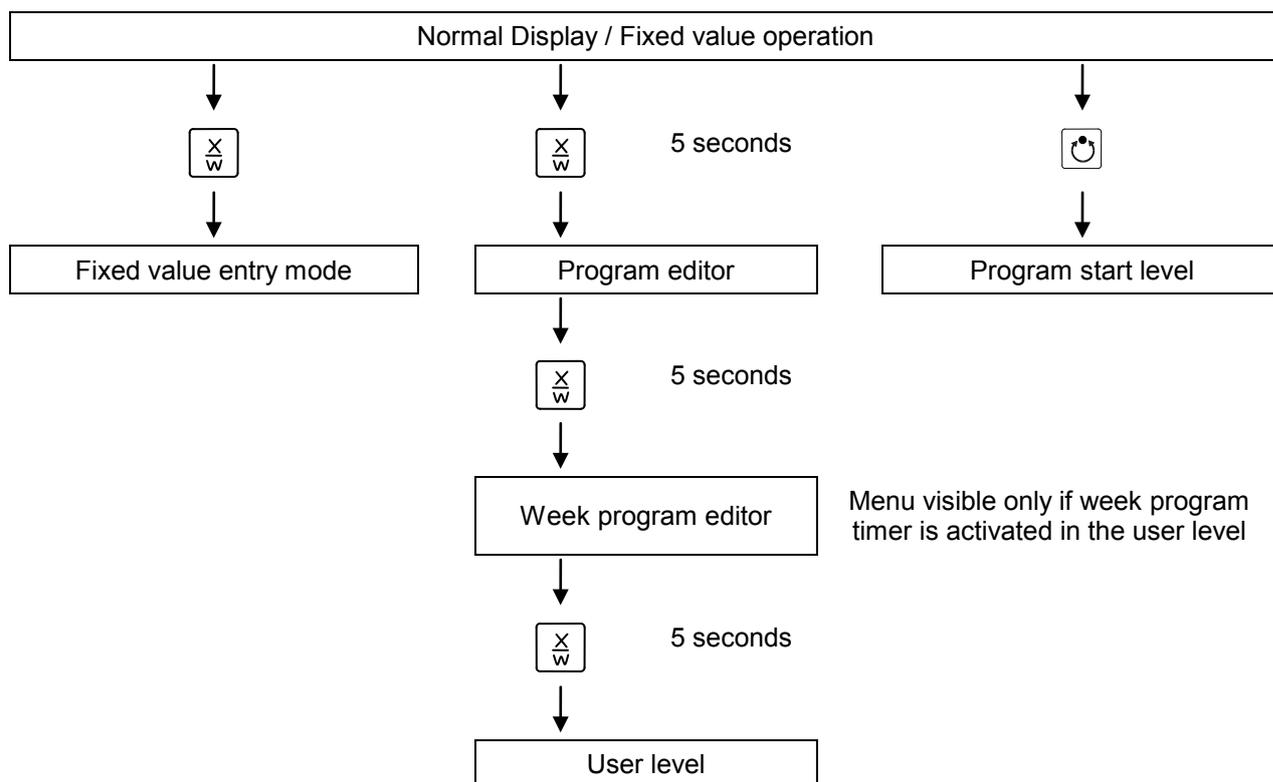
If no button is touched during more than 120 sec. the controller returns from the actual level to Normal Display.
