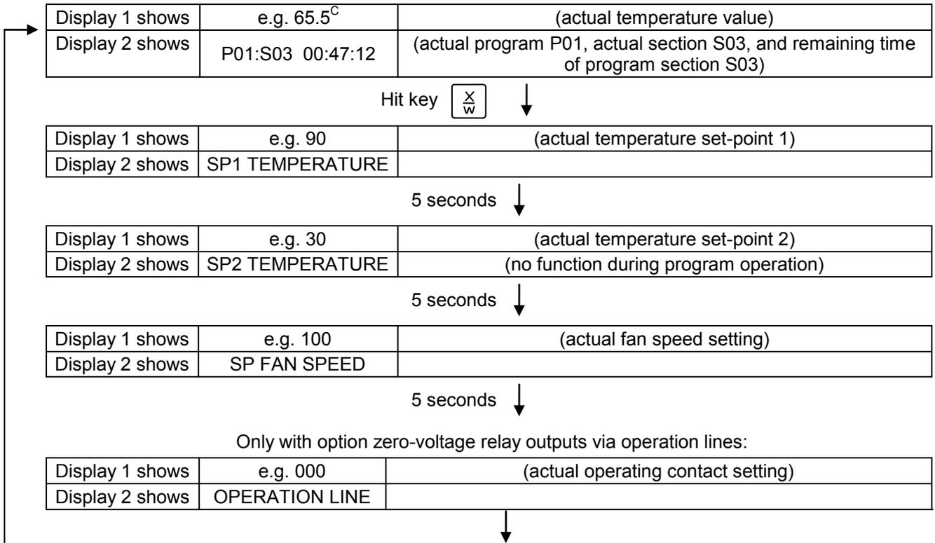
After program runoff (and, if appropriate, of the program repeats) the controller returns to fixed value operation showing Normal Display and adjusting to the temperature and fan speed values that have been previously entered in the fixed value entry mode.
