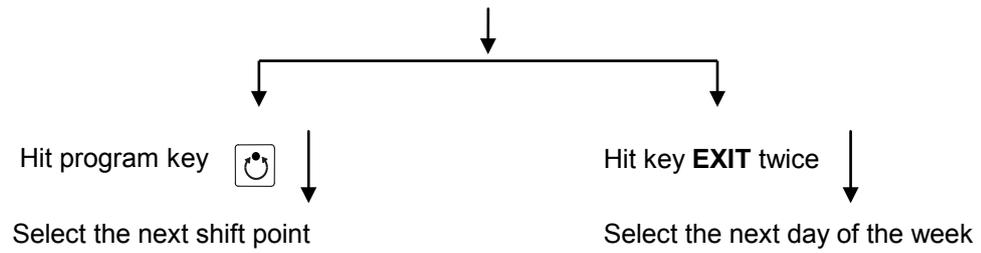
To exit the menu, hit several times key EXIT or wait for 120 seconds. Controller returns to normal display.
