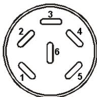
Figure 13: Pin configuration of the DIN socket
