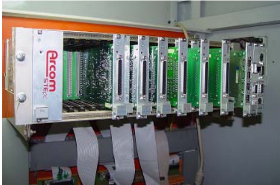
Figure 4: STePc with single board computer and I/O cards
