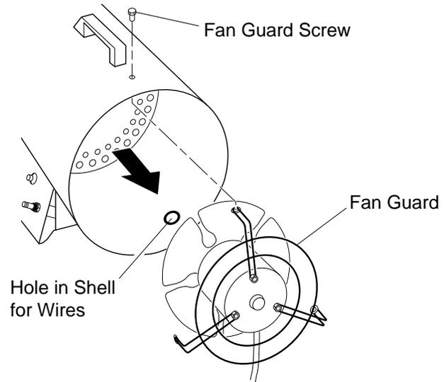
**Figure 7 - Removing Motor and Fan Guard from Heater**
