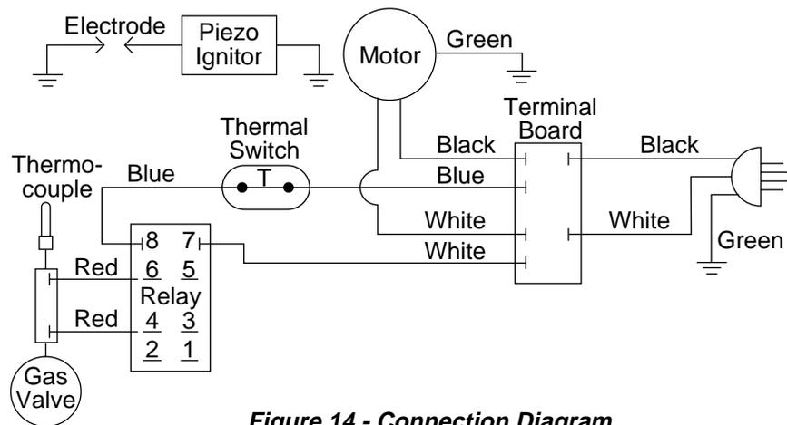
**Figure 14 - Connection Diagram**
