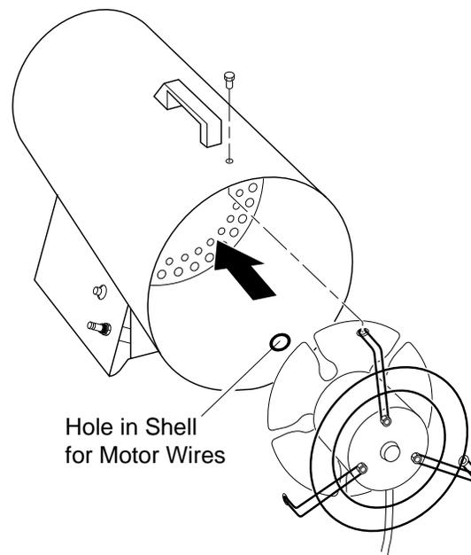
**Figure 10 - Replacing Motor and Fan Guard into Heater**
