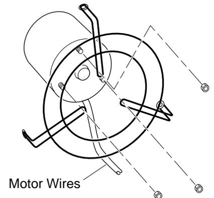
**Figure 9 - Removing or Attaching Fan Guard from Motor**
