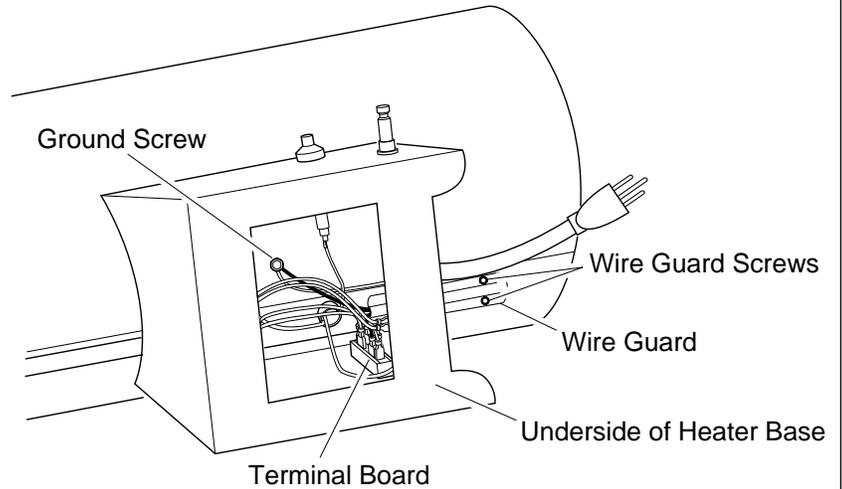
**Figure 6 - Location of Ground Screw and Wire Guard**
