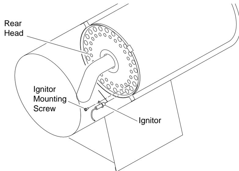
**Figure 12 - Removing Ignitor Mounting Screw and Ignitor**
