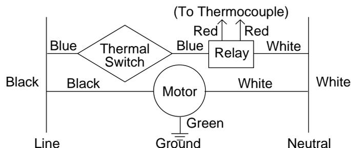
**Figure 15 - Electrical Ladder Diagram**
