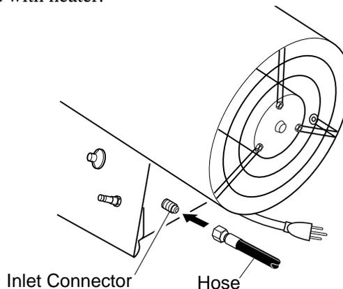
**Figure 4 - Hose and Inlet Connector**
