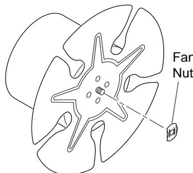
**Figure 8 - Removing Fan Nut from Motor Shaft**
