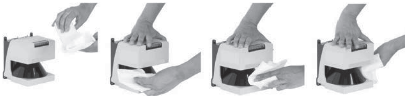
Fig. 11.8-1: Cleaning the optical window
