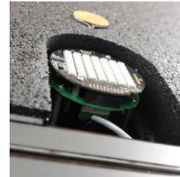
5. Place panel #P1B above panel #P1A and bring it into place making sure that the cable connection at the top of #P1A can fit through the hole located at the bottom of #P1B so that it can later connect with the target just above the hole on panel.
