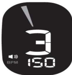
1. Press and hold **MODE/TUNING ITEM/BEAT** button for 2 seconds to switch between tuning mode and metronome.
