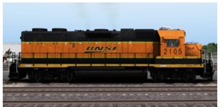
EMD GP38-2, BNSF Rebuild
