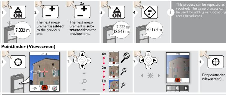
This is a great help for outdoor measuring. The integrated pointfinder (viewscreen) shows the target on the display. The device measures in the middle of the cross hair, even if the laser dot is not visible.
