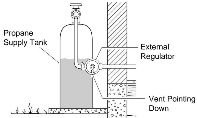
Figure 13 - External Regulator With Vent Pointing Down
