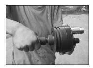
**Step 3 Remove Bearing Plate** – The bearing plate and sealing plate are connected by two interlinking screws. Unthread these screws with a hex wrench.
