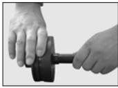
**Step 4 Assemble Feed/Concentrate Port** – Place the feed/concentrate port in the sealing plate opening and secure using the two feed/concentrate port fixtures.
