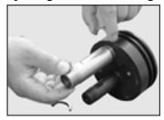
**Step 5 Assemble the Bearing Plate** – Position the bearing plate over the sealing plate, pushing them together so that the threaded portion of the permeate port is visible. Connect the bearing plate and sealing plate with the two interlock screws. A hex wrench can be used to secure the screws.
