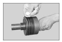
**Step 2 Remove Adapter** – Grasp the adapter and slowly pull from the bearing permeate port. A slight rotating motion may ease the removal of the adapter. There is a set of double o-rings on the inside diameter of the permeate port that must be inspected for damage once the adapter is removed. Damaged o-rings must be replaced before re-installation.
