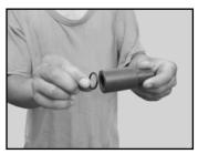
**Step 7 Install Adapter** – The adapter should be pushed into the permeate port until the wider diameter middle section is flush against the end of the permeate port. Simultaneously pushing and turning the adapter will ease installation.
