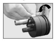
**Step 4 Remove the Feed/Concentrate Port** – Remove the two pieces of feed / concentrate port fixture. Grasping the sealing plate, rock the feed/concentrate port slightly and pull away from sealing plate. It may be necessary to tap the permeate port on the smaller end with a rubber mallet to release the seal bond.
