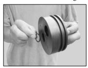
**Step 3 Assemble Permeate Port** – Install the permeate port into the sealing plate.
