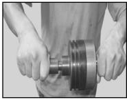
**Step 8 Install Head O-ring -** All o-rings should be coated with a thin layer of glycerine before installation. Seat the head o-ring into the groove on the outside diameter of the head.
