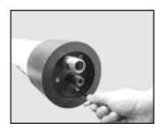
**Step 5 Remove the End Plug** – A male threaded nipple is recommended for use when opening the end plug. Thread the pipe nipple into the permeate port of the end plug, gently motion the nipple in various directions, and then gently pull the nipple from the vessel. A firm tug may be required to release the end plug o-ring seal.
