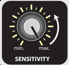
If the detector emits false signals due to interference, reduce the sensitivity until the signals go away and start searching.
