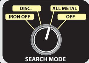
To turn on the device, rotate the search mode knob to the desired mode. Turn the same knob to OFF position to when you want to turn off the device.
