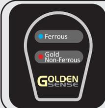
When the device detects a metal, it will produce an audible tone. If the device is in discrimination mode, the LEDs on the handle will light up at the same time.
