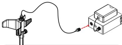
Plug the other end of the system connection cable into the coil input socket underneath the system box and tighten securely.
