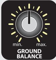
Rotate the sensitivity knob to maximum and the ground balance knob to the mid-level.
