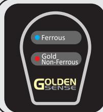
When the device is turned on, a melody will be heard and both LEDs on the handle will light up. Approximately 20 seconds later, the LEDs on the handle will go off and you will hear a tone indicating that the device is ready to use.
