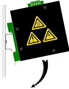
To install the unit to 35mm industrial DIN-Rail, place the top edge of the included mounting bracket on the back of the unit against the DIN-Rail at a 15° angle as shown. Rotate the bottom of the unit to the back (away from you) until it snaps into place.
