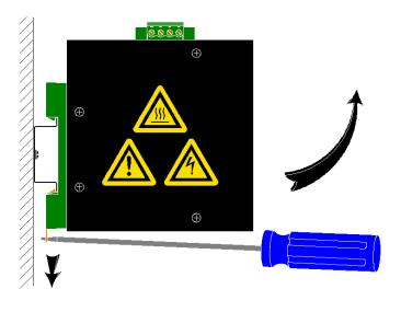
To remove the unit from the 35mm industrial DIN-Rail, place a flat head screwdriver into the orange release clip found at the bottom of the unit, and apply downward force on the clip until it disengages from the bottom of the unit from the DIN-Rail. Rotate the bottom of the unit towards you and up at an approximate 15° upward angle to completely remove the unit.
