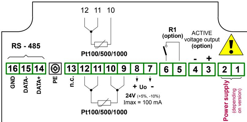
Figure 4.10. Terminals description (relay and active voltage outputs)
