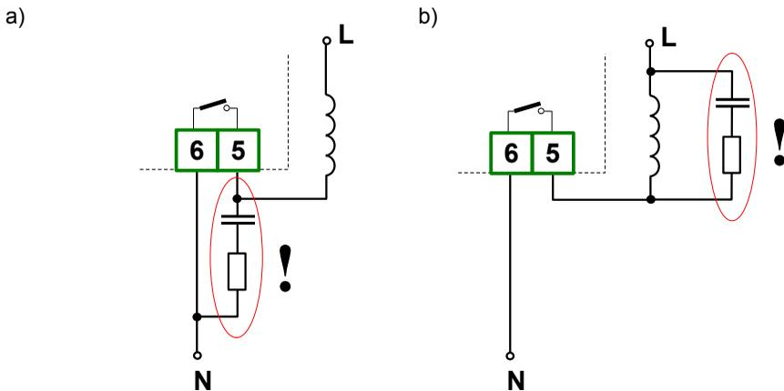
Figure 4.14. Examples of suppression circuit connection:
