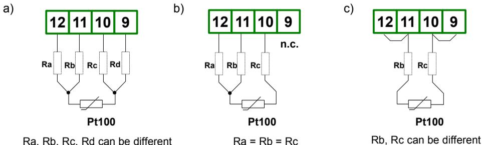
Figure. 4.12. Connection of sensors:
