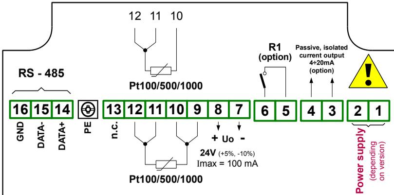
Figure 4.8. Terminals description (relay and passive current outputs)
