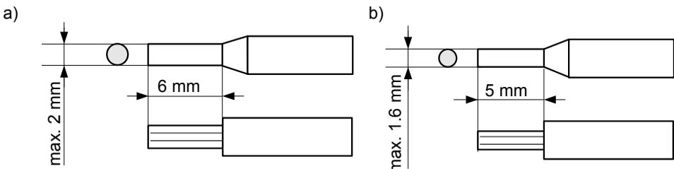
*Figure 4.2. Recommended dimensions of cable stripping
