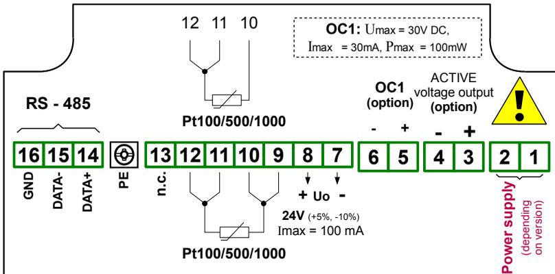
Figure 4.11. Terminals description (OC-type and active voltage outputs)
