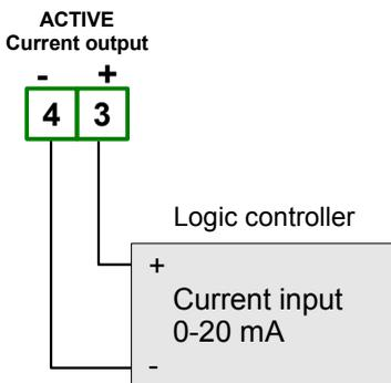
Figure 4.16. Example of active current outputs connection
