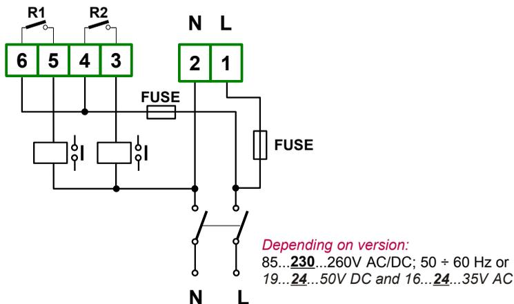
Figure 4.13. Connection of power supply and relays
