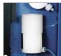
Reagent mixing chamber allows automated online reagent blending in the method
