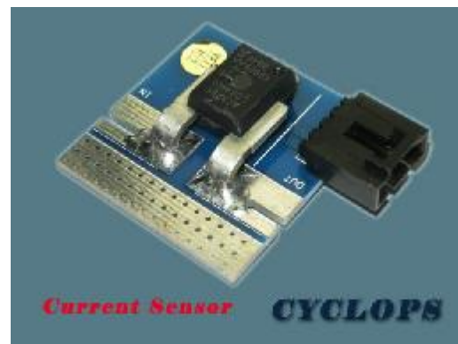
Voltage and current sensor(50V、100A)(11g)
