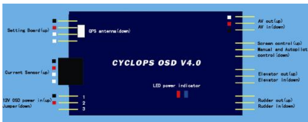
Current sensor connection diagram
