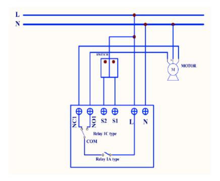
Place the in-wall switch into a wall box and connect the pins as shown in the figure.
