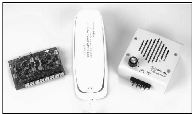
Fig. 3 - Accessories for Order-Wire include active 4w/4w bridge, 4-wire DTMF phone and speaker.
