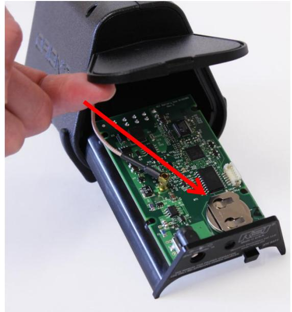
Note: The provided internal coin cell is a CR2032 battery with the following specifications: 3V nominal voltage, 225 mAh nominal capacity, -30°C to 60°C operating temperature.
