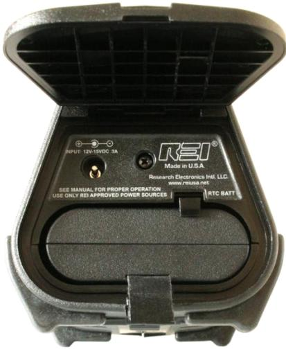
To insert or switch out a new battery:
