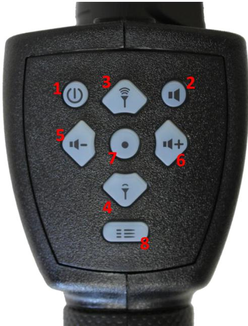
1. **POWER** – Press to Power on. Press and hold while the unit is on to Power off. A quick press of the power button while the unit is on will toggle the Transmit Power Mode (Auto or Manual)
