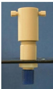
**Figure 15: Pressure relief valve**
