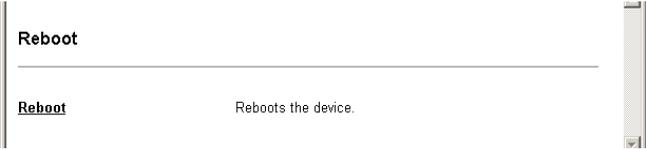
Once all parameters have been set and saved by clicking on each tabs "OK" button, the Barix Barionet needs to be restarted to use the new settings. This can be achieved by simply switching the unit off and on again, or conveniently from the web interface. The reboot typically takes no longer than 10 seconds, however, be aware that your browser will time out if you changed the IP address:
