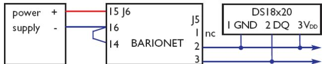
2.) Use the included extension cable (2 x 3 pin connectors, red, black and white cable) and connect 1 wire to pin 3 (white cable) and the other cable to the digital output ground. This way is recommended by Barix for being more reliable and more resistant to electromagnetic disturbances.
