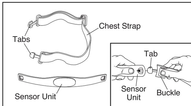
Insert the tab on one end of the chest strap into the hole in one end of the sensor unit, as shown in the inset drawing above. The tab should be flush with the front of the sensor unit.
