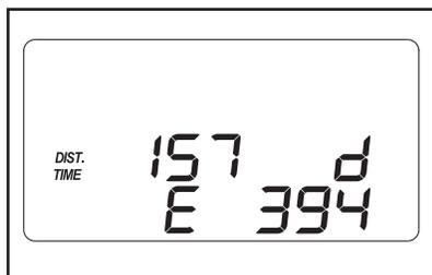
In addition, an “E” for English miles or an “M” for metric kilometers will appear in the lower left corner of the display. To change the unit of measurement, press the Speed increase button.
