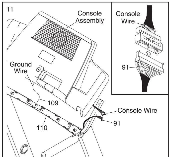
12. Set the console assembly on the Left and Right Uprights (77, 92). **Be careful not to pinch any wires.**
