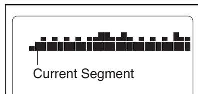
profile represents the current segment of the workout. The height of the flashing segment indicates the speed setting for the current segment. At the end of each segment, a series of tones will sound and the next segment of the profile will begin to flash. The new speed and incline settings will appear in the display and the treadmill will automatically adjust to the new speed and incline settings.
