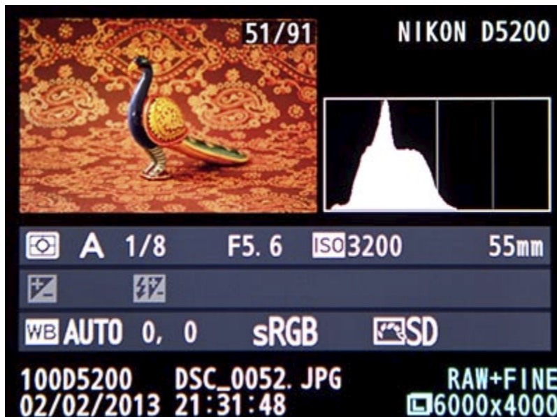
Figure 17 - The Overview information display screen during image playback, showing a thumbnail of the image along with the RGB Histogram and shooting and file information.
