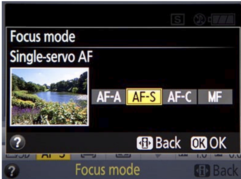
Figure 84 - Single-Servo AF Focus Mode, AF-S, as accessed on the Information Display screen.
