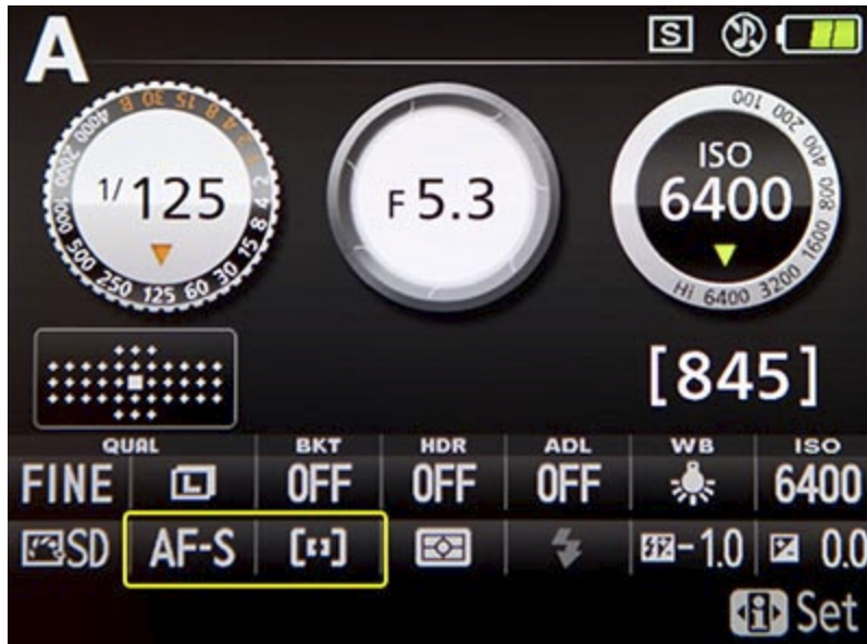
Figure 83 - Selecting the Focus Mode and AF-Area Mode on the Information Display Screen. These two settings are shown circled in yellow here.
