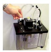
Press clear tubing firmly into white fitting.
