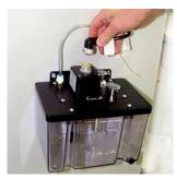
Attach black power cable to power fitting.
