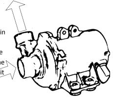
**Attention:** Please only mount the pump with appropriate rubber dampers because high vibration can damage the internal electronics!
