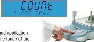
Utilizing the 2-line LCD, SmarText simultaneously displays weight and application specific information such as percent or count. For example, with one touch of the Function button, SmarText will display application reference information such as average piece weight (APW), while displaying a parts count.
