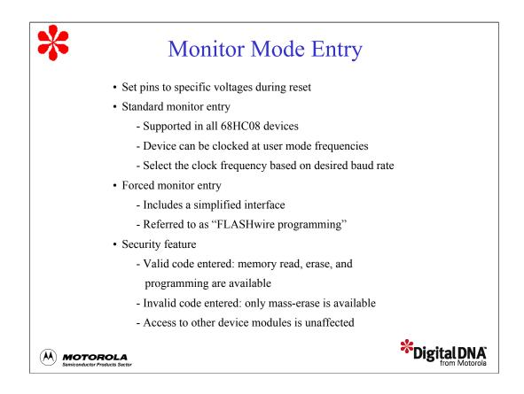
In-circuit programming is the preferred method for programming a blank part. Although the monitor is a very simple device, you must satisfy all entry conditions to access it. These conditions are satisfied by setting the pins to specific voltages during reset. The two ways to enter monitor mode are standard monitor entry and forced monitor entry.
