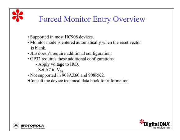
Most of the newer HC908 devices support forced monitor entry. With this entry method, the part automatically goes into monitor mode when the part is blank, indicated by a blank reset vector. This eliminates the need to apply a high voltage to IRQ and the need to satisfy port conditions for monitor entry. Keep in mind that there may be additional port pin requirements to make the monitor operate the way you want. For specific information, consult the device technical data book.
