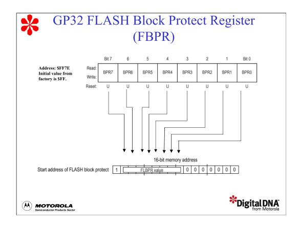
Now that we've reviewed the procedures for programming and erasing FLASH, let's discuss another important concept called FLASH block protection. Block protection enables you to protect an entire array, or a portion of an array, from being erased or reprogrammed. This protection is implemented using the FLASH block protect register (FLBPR), itself a FLASH location.
