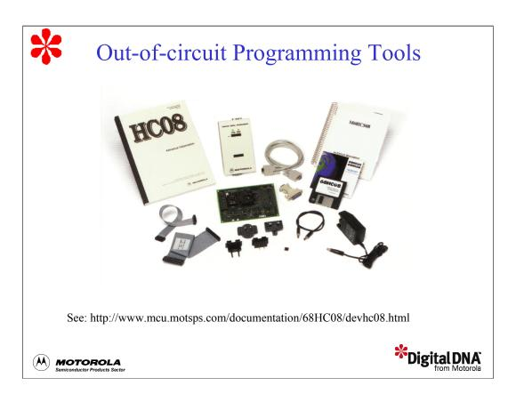
The easiest method to program a blank part is out-of-circuit programming. With this method, you don't have to follow programming procedures or satisfy monitor mode entry requirements. The programmer takes care of these details. To program out-of-circuit, simply connect your device to the programmer, load the s-record file, and then press a button. Your device will be programmed in a matter of seconds.
