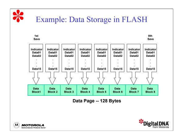
Suppose you have 15 bytes of parameters that you want to maintain in non-volatile memory and modify as needed. Let's also suppose that you are using the 68HC908GP32 controller. In this controller, a 128-byte page is the smallest erase block.
