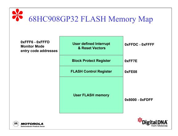
Let's look next at how FLASH memory is organized. FLASH memory in 68HC08 MCUs is usually an array of either 8192 or 32,768 eight-bit bytes. The FLASH array is always mapped at the top of the 64k memory map. This means that an 8k array is mapped from \$E000 to \$FFFF. The figure shows the 68HC908GP32 32k array in which FLASH is mapped from \$8000 to \$FFFF.
