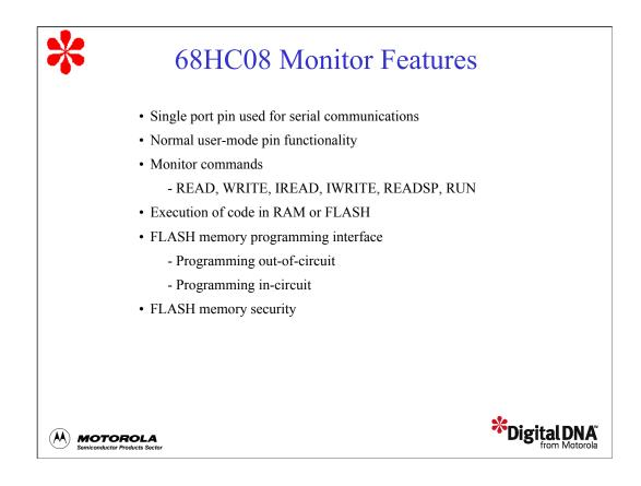
Next, let's discuss entering and using monitor mode beginning with an overview of the monitor features. Monitor mode is available on all 68HC08 devices. Monitor mode is primarily used to provide serial access to the device and its internal modules for programming, reading, debugging, and testing activities. You must use this mode to program a blank device. This is accomplished on a single port pin while still retaining all other user mode pin functionality.
