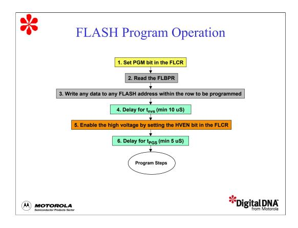
The FLASH program procedure is a 13-step operation. The figure shows the first six steps. As you can see, the program procedure is similar to the erase procedures.
