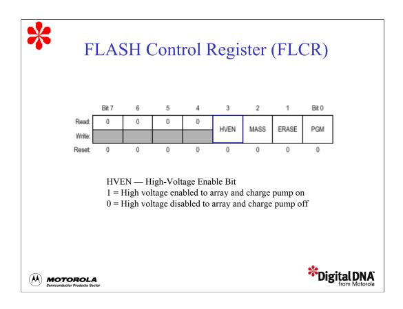
The FLASH control register, FLCR, is usually located at address \$FE08 and consists of four bits that enable you to program or erase FLASH.
