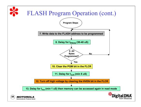
Another difference between this procedure and the erase procedures is the loop in steps 7-9. In the loop, we write a byte of data to the desired address, delay, and then verify that all of the bytes have been programmed. This process is repeated until we finish writing all of the locations we want to program.
