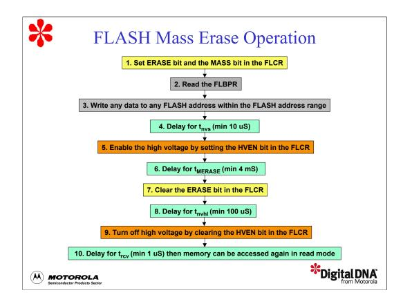
The procedure for erasing the entire FLASH array is similar to the page erase procedure, with a few differences.
