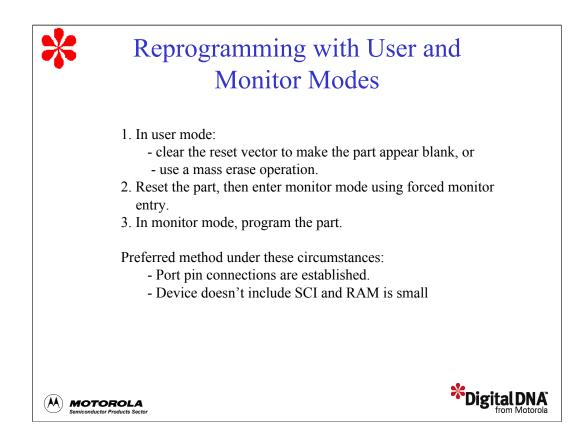
The next method for reprogramming a device in-circuit involves performing operations in both user mode and monitor mode. For devices that support forced monitor entry, it may be advantageous to first make the part blank, or appear blank, in user mode. Then, you can use forced monitor entry to program the part.
