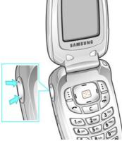
In Idle mode, you can also adjust the keypad tone volume using these keys.
