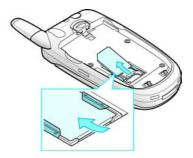
5. Place the battery so that the tabs on the end align with the slots at the bottom of the phone.
