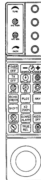
Fig.21 Front Panel Controls
