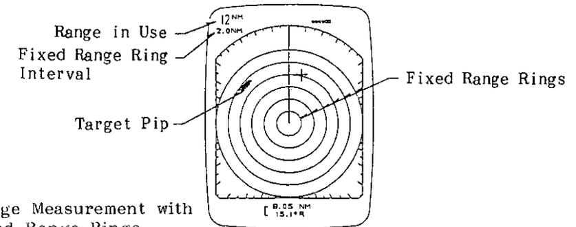
Fig.25 Range Measurement with Fixed Range Rings
