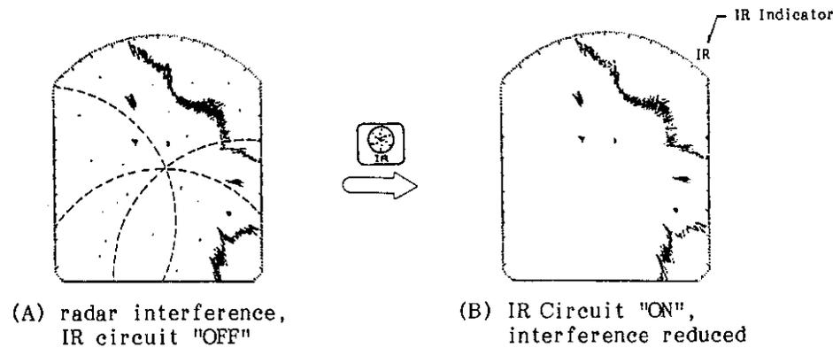
Fig.29 Radar Interference
