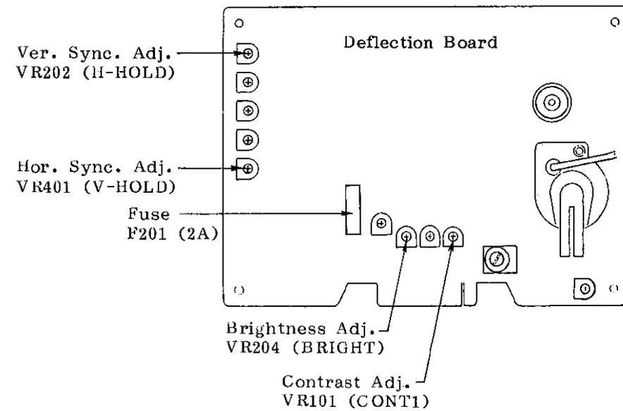
Note: Since the CRT is turned 90°, the indications "V" and "H" correspond to "horizontal" and "vertical", respectively.
