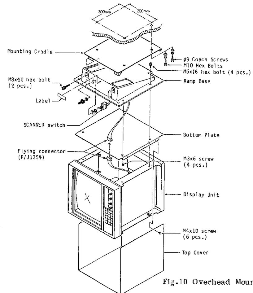
Fig.10 Overhead Mounting
