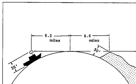
Fig.38 Radar Horizon
