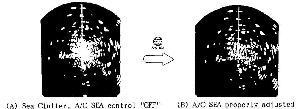
Fig.24 Adjusting the A/C SEA
