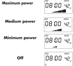
At any time during "Manual" operation, pressing the "ON MODE" button once will display the previously set power level for 5 seconds; after this 5 second period, the display will return to show the current operating power.
