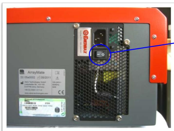
Main POWER switch & power supply cable inserted in appropriate line connector
