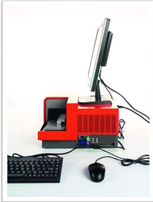
*fig. 3: right side with connector board for monitor, PS/2, serial, USB and other interfaces*
