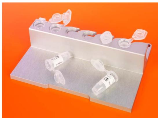
fig. 12b: incorrectly placed ArrayTubes
