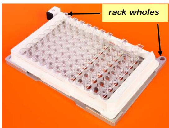
fig. 11a: ArrayStrip rack with inserted strips and rack wholes for position rack into rack fitting. Ensure correct insertion of strips by slightly pressing them into strip frame.
