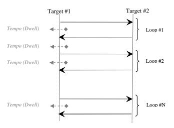
In the "Target position / PA-Move Absolute" area, two target positions can be defined. The "Go to" button allows executing the absolute move to go to the specified target position.
