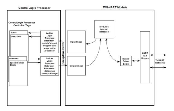
All data transferred between the module and the processor over the backplane is through the input and output images. Ladder logic must be written in the ControlLogix processor to interface the input and output image data defined in the controller tags. The user is responsible for handling and interpreting all data received on the application ports and transferred to the input image.
