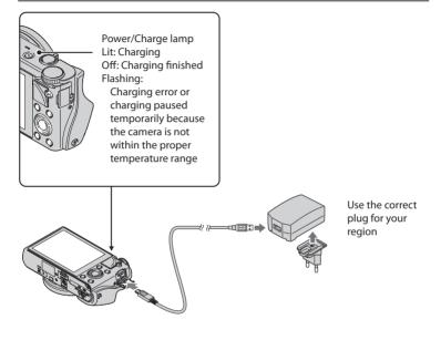
1 Connect the camera to the AC Adaptor (supplied), using the micro USB cable (supplied).
