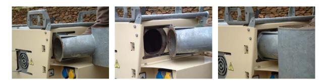
The bagging unit attaches to the front access panel of the power unit
