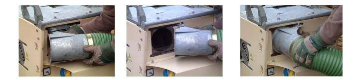
The 150mm Blower hose connects to the outlet access panel, on the main power unit.
