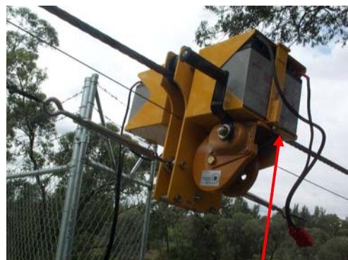
Locking pin used to hold battery and winch in place
