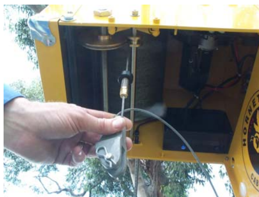
Lower the cable to attach the C1 Connector to the Hanger Bar
