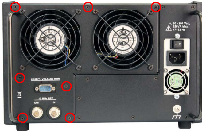
FIGURE 5-5 - REMOVING THE FANS STEP 1
