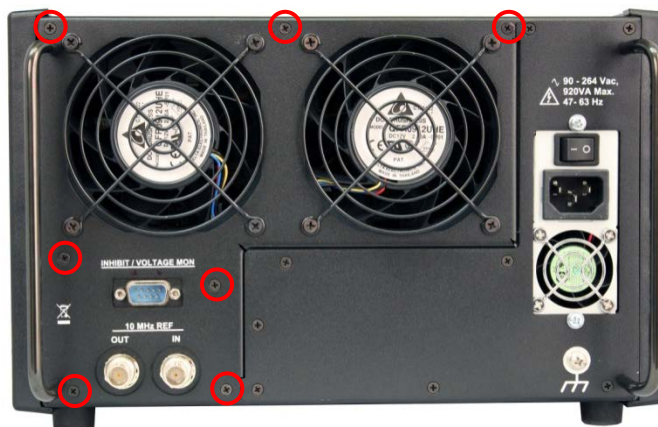
FIGURE 5-11 - REINSTALLING THE FANS STEP 3
