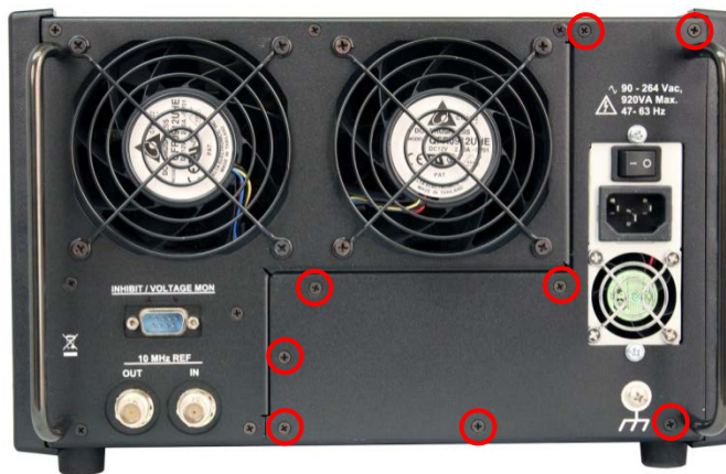
FIGURE 5-1 - REMOVING THE POWER SUPPLY STEP 1
