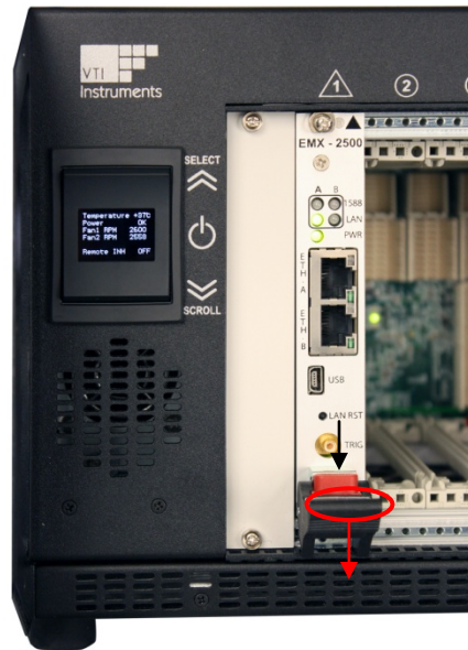
FIGURE 3-6 - PLUG-IN MODULE REMOVAL STEP 2
