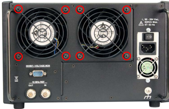
FIGURE 5-9 - REINSTALLING THE FANS STEP 1
