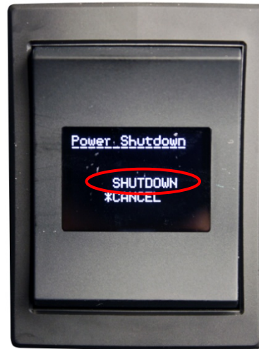
FIGURE 4-20 – FRONT PANEL SHUTOFF
