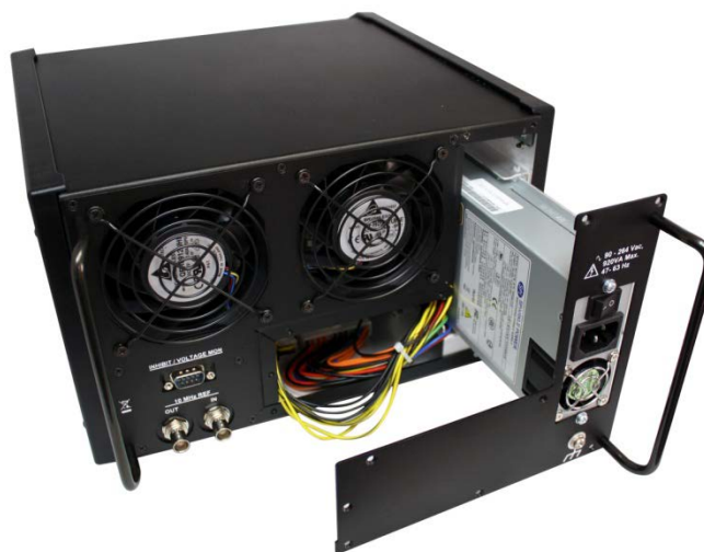
FIGURE 5-2 - REMOVING THE POWER SUPPLY STEP 2
