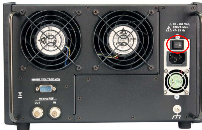
FIGURE 4-21 – REAR PANEL SHUTOFF
