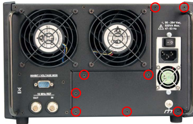
FIGURE 5-15 - REINSTALLING THE POWER SUPPLY STEP 7
