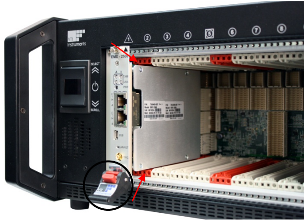
FIGURE 3-2 - PLUG-IN MODULE INSTALLATION STEP 1
