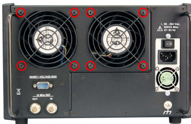
FIGURE 5-8 - REPLACING THE FANS STEP 4
