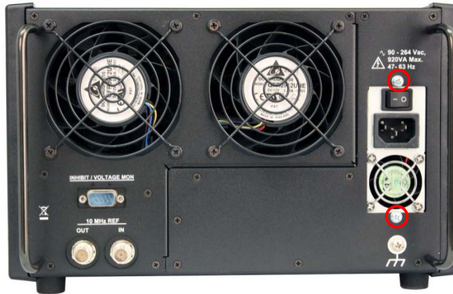
FIGURE 5-12 - REINSTALLING THE POWER SUPPLY STEP 4
