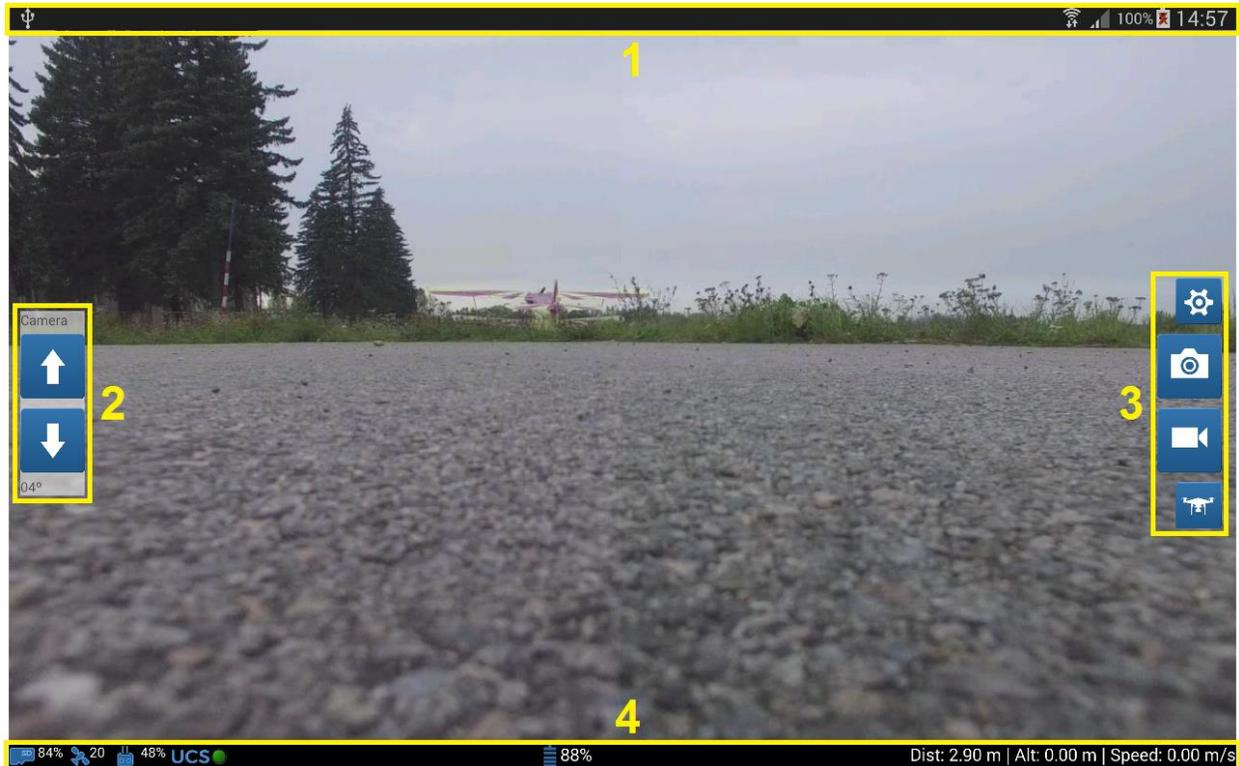
Main application screen could be divided in four zones, as shown on image: system bar (1), camera position control panel (2), vehicle control panel (3) and application status bar (4).
