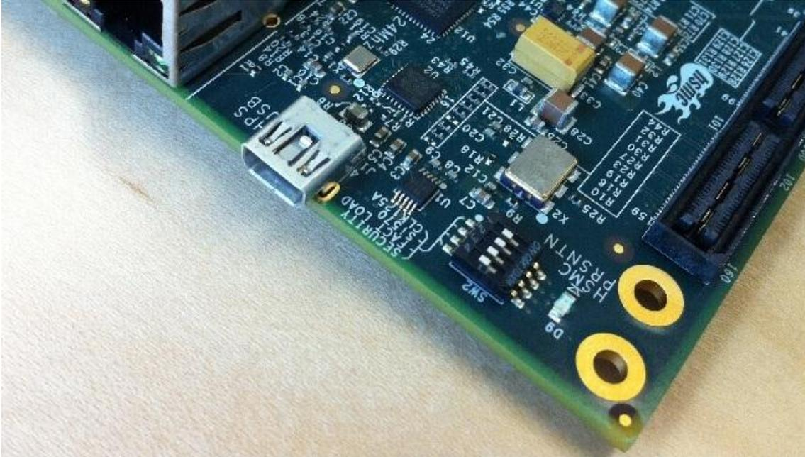
3. Use a mini-USB to USB cable to connect “UART” on the board to the host PC (May need to install Cypress UART-to-USB driver)
