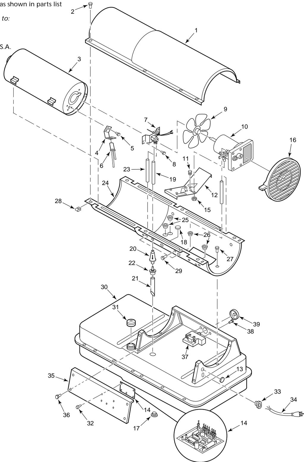
**Figure 33 - Replacement Parts Illustration for Model 3E218E**
