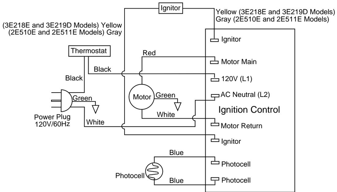
Figure 36 - Wiring Diagram for All Models
