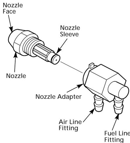
**Figure 22 - Nozzle and Nozzle Adapter, All Models**
