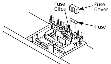
**Figure 28 - Replacing Fuse**
