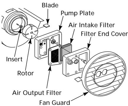
**Figure 25 - Rotor Location, Models 3E218E and 3E219D**
