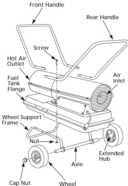
Figure 6 - Wheel and Handle Assembly, Models 3E218E and 3E219D Only
