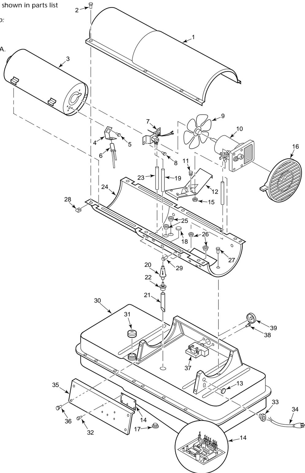
**Figure 34 - Replacement Parts Illustration for Model 3E219D**
