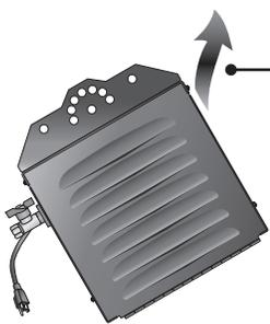
Discharge released from side air channels. Keep area clear of gas piping and electrical wiring.
