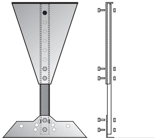
**Figure 2.6 - Typical Side Wall Mounting**
