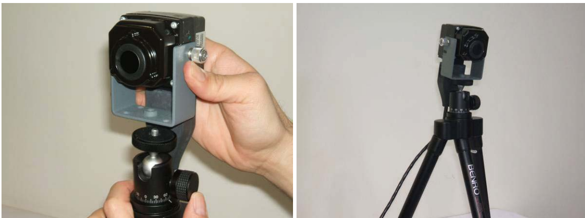
Figure 11: Attaching Mini-Thermal to Tripod
