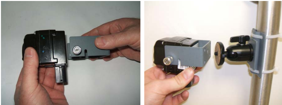
Figure 16: Installing Mini-Thermal Camera to Bracket
