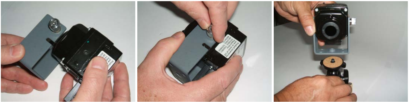
Figure 6: Attaching Mini Thermal Camera to Mounting Bracket
