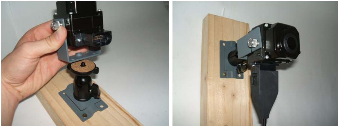
Figure 14: Mounting Mini-Thermal Camera to Wall
