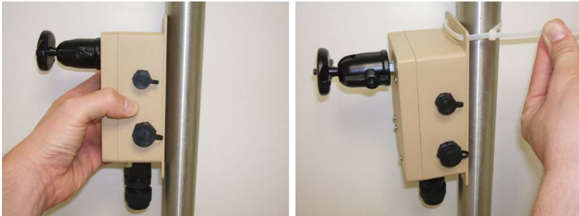
Figure 5: Pole Mounting DOG Remote Module
