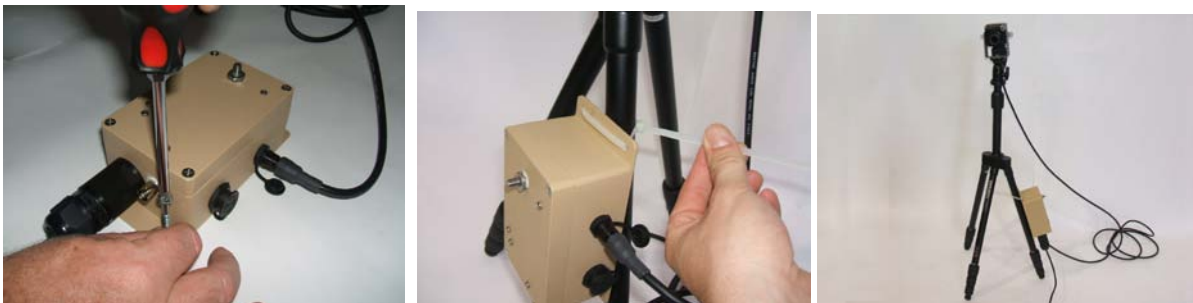
Figure 19: Mounting the DOG Remote Module
