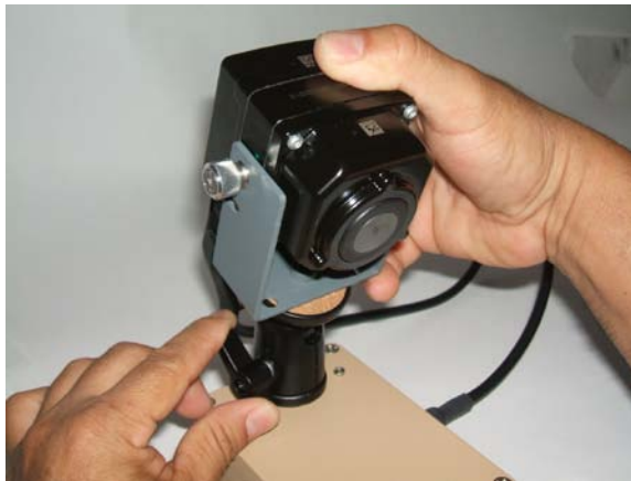
Figure 8: Adjusting the Camera's Tilt and Rotation
