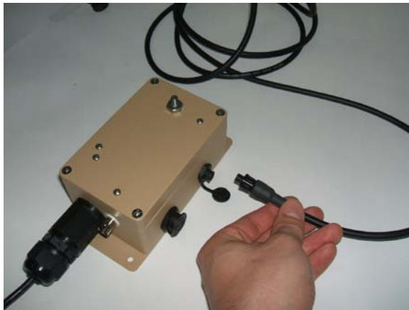
Figure 18: Connecting Mini-Thermal to DOG Remote Module
