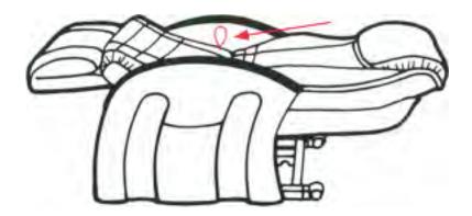
For Zero Gravity position, start with the chair in it's normal upright position and pull the looped cord on the right side of the chair between the seat and arm up and forward, the cable will appear slightly shorter. This will lock the chair into the Zero Gravity position.
